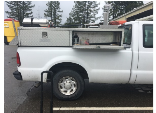
Utility Bed on Pick-up Bottom of Storage at 55" from ground- Herbicide and Chainsaws stored here
