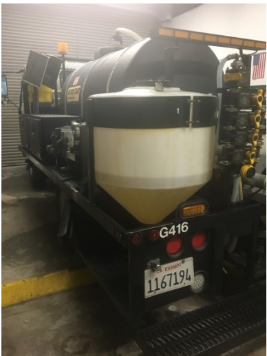
Tank of Herbicide- Top of tank At 64" from floor; 46" from step
