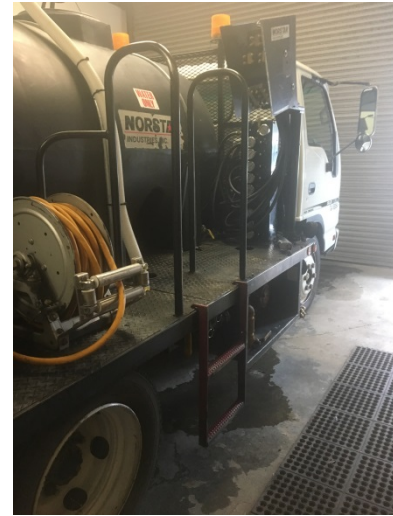
Side of Spray/Tank Truck- Portable Ladder Steps at 12" – 24" – 36" to bed of truck
