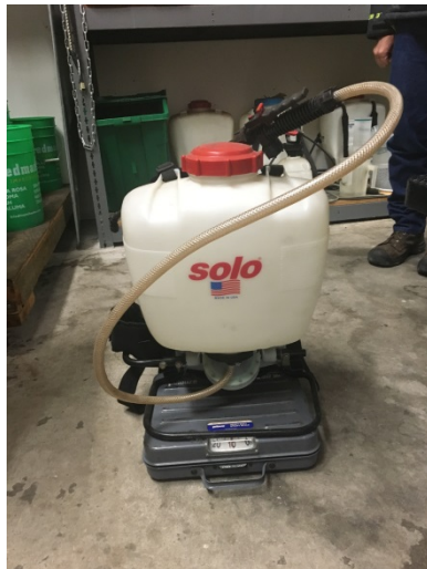
4 Gallon Spray Back Pack- (Typically filled with ONLY 3 Gallons) Empty- 10 lbs.; Plus 3 Gal. - 35 lbs. ; Plus 4 Gal. – 43 lbs.
